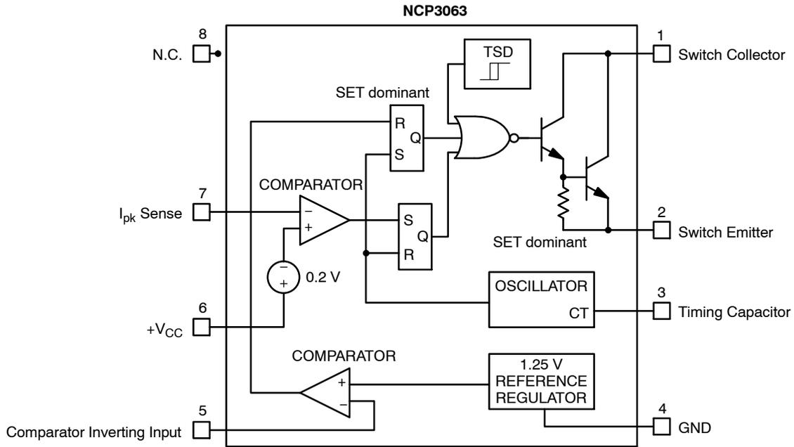
Figure 4. Block Diagram
