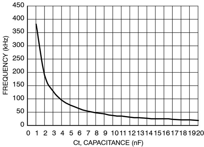
**Figure 5. Oscillator Frequency vs. Oscillator Timing Capacitor**
