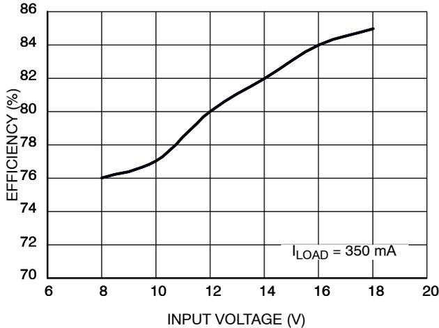
**Figure 26. Typical Efficiency for Application Shown in Figure 25.**
