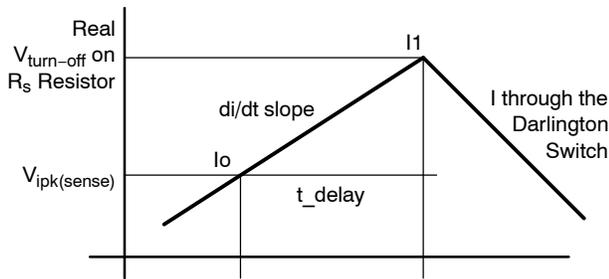
The  $V_{IPK(Sense)}$  Current Limit Sense Voltage threshold is specified at static conditions. In dynamic operation the sensed current turn-off value depends on comparator response time and di/dt current slope.
