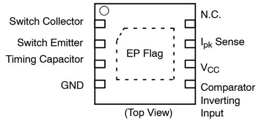
NOTE: EP Flag must be tied to GND Pin 4 on PCB
