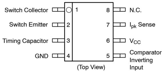
Figure 2. Pin Connections
