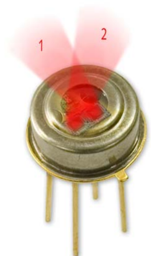
Figure 21: identification of zone 1&2 relative to alignment tab.
