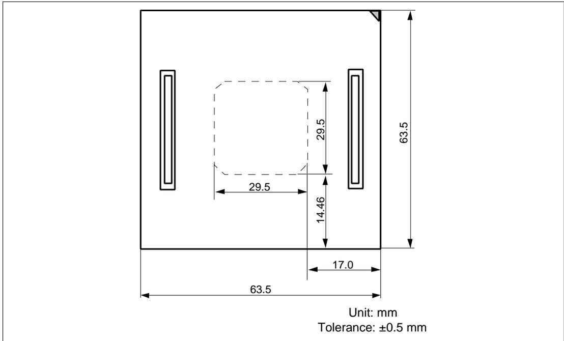
**Figure 6 Dimensions for User System Interface Cable Head**
