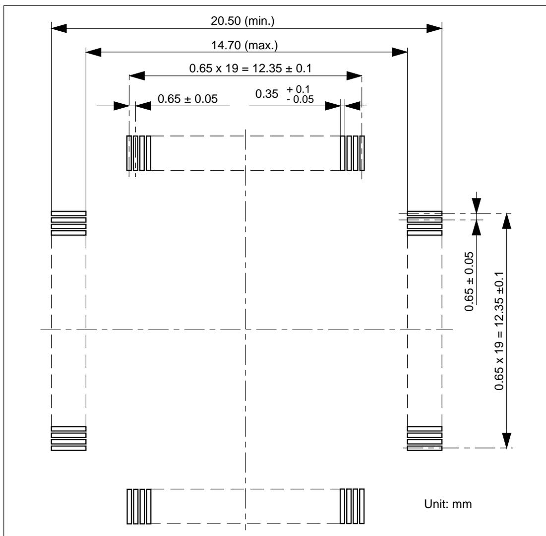
Figure 5 Recommended Dimensions for Mount Pad
