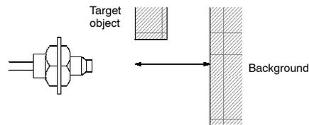
Keep an appropriate distance between the sensor and the background object. The background surface should be covered with a material that has a small reflection factor, such as a black sponge sheet.
