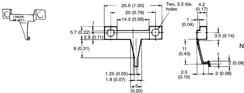
Note: Use the EE1003A Connector Holder to prevent accidental disconnection of the EE-1003 Connector from the EE-SPZ301/401 Photomicrosensor.
