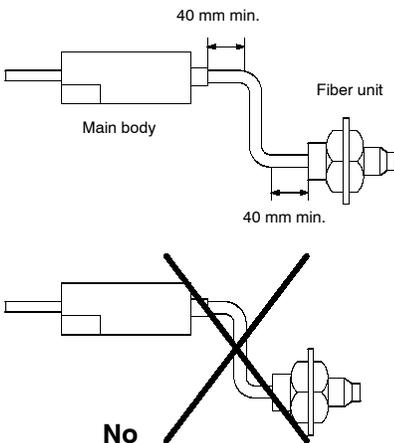
Install the Fiber Unit with nylon cable holders or cable ties as shown below so that no excessive force is directly applied to any section of the cable.
