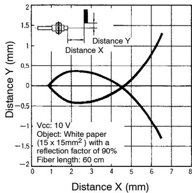
**FIBER LENGTH VS. RELATIVE SENSING DISTANCE (TYPICAL)**
