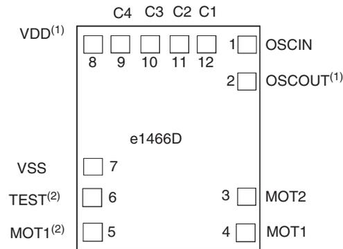
(1) The pads VDD and OSCOUT are interchangeable per mask option
