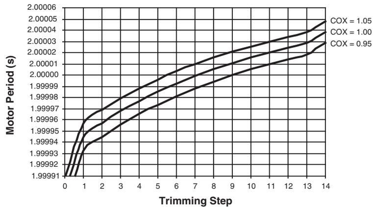
COX means frequency deviation due to production process variations.
