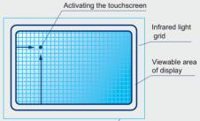
The infrared light beams emitted by LED Pairs form a invisible grid on the glass
