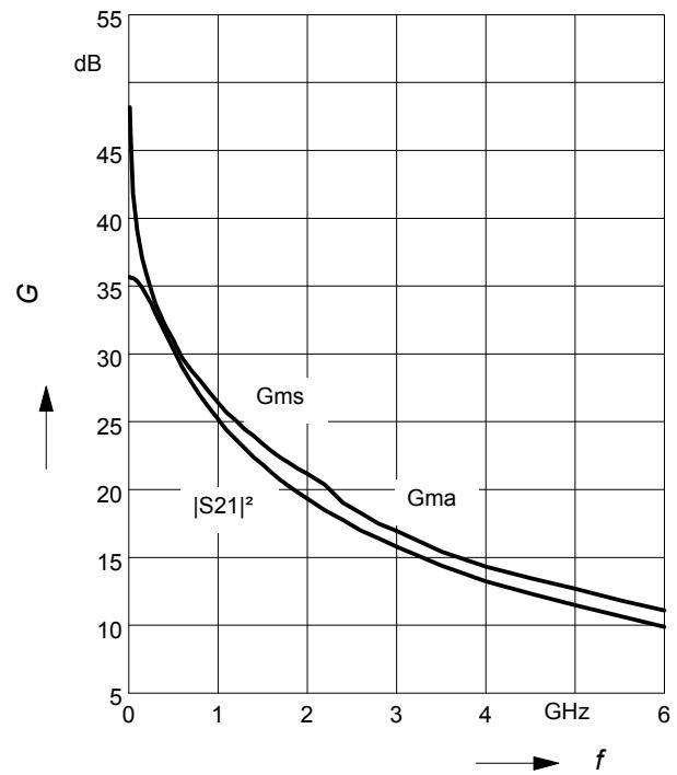
**Power gain  $G_{ma}$ ,  $G_{ms} = f(V_{CE})$**
