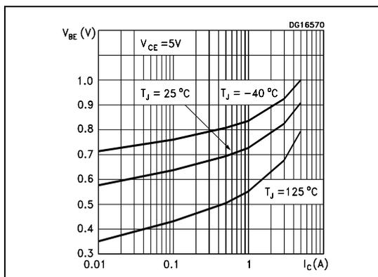
Figure 7. Base-emitter voltage
