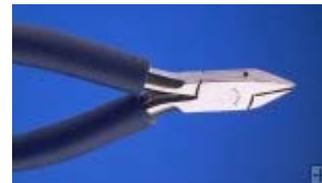
[4 1/2" Standard Tapered Head Cutter, Flush](#)
