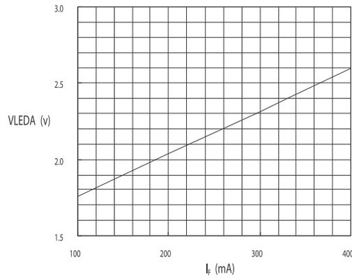
Figure 4. I<sub>F</sub>-VLEDA Characteristics (0°)
