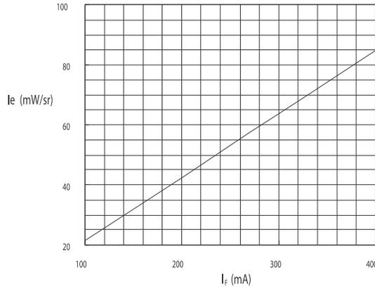
Figure 3. I<sub>F</sub>-I<sub>e</sub> Characteristics (0°)
