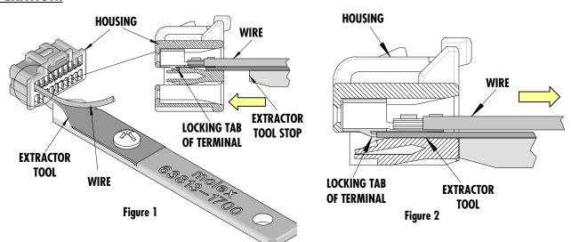
Push the terminal and the wire forward in the arrow direction before using the Extractor Tool. Insert the Extractor Tool into the slot below the terminal until the stop on the tool contacts the plastic housing as shown in Figure 1. This will flex the plastic lance freeing the terminal.
