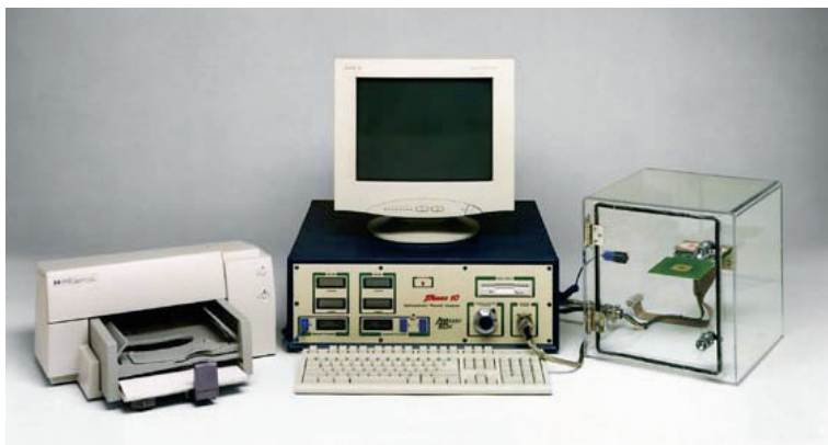
Figure 3-4: \theta_{JA} Measurement Setup
