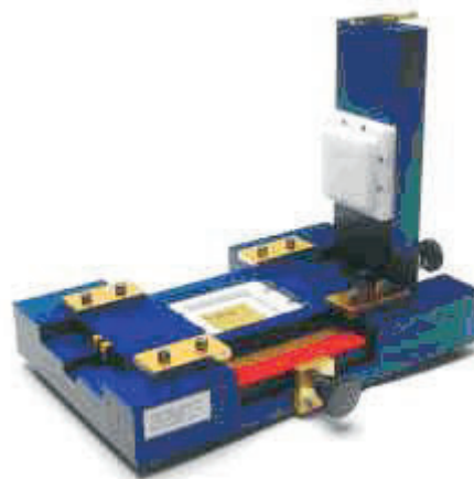
Figure 4-1: Altair BGA Fixture Used for TDR Measurement
