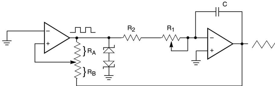
frequency  $\propto R_1, R_2, C$
