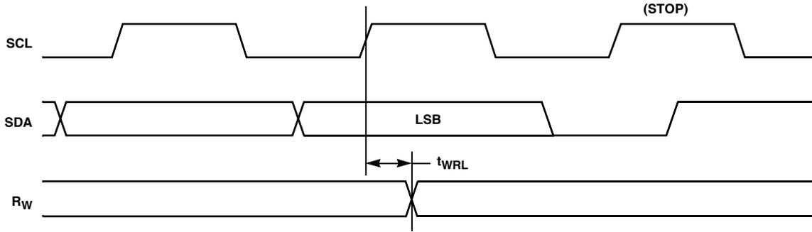
**Write Protect and Device Address Pins Timing**
