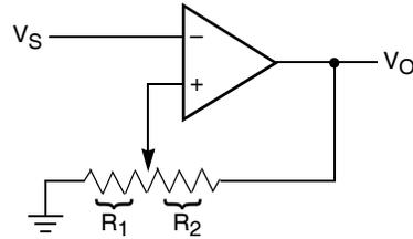
$$V_{UL} = \{R_1/(R_1 + R_2)\} V_O(\text{max})$$
