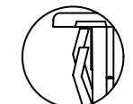
DETAIL VIEW VH1 HOLE PLUG (No wing serrations for ease of removal)
