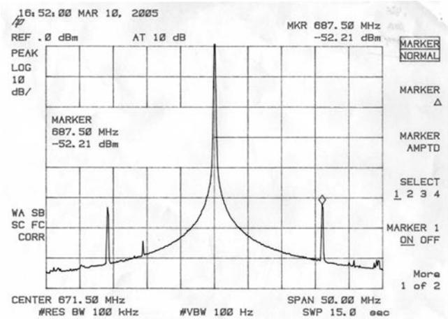
**Figure 4b. Reference Spur at -52dB at 16MHz**
