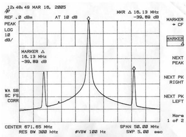
**Figure 4a. Reference Spur at -39dB at 16MHz**
