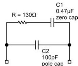
Figure 3a. Loop Filter for Lowest Cycle-to-Cycle Jitter
