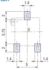
Note) The zero point is the center of mounting.
