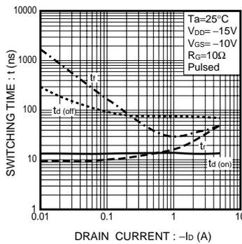
Fig.8 Switching Characteristics
